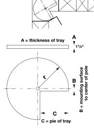
Adjustable post fits 23 <sup>1</sup>/4" - 33" high cabinets. Material: Shelves: high impact polystyrene Post: steel, chrome-plated Bearings: nylon Bottom support: steel, galvanized
